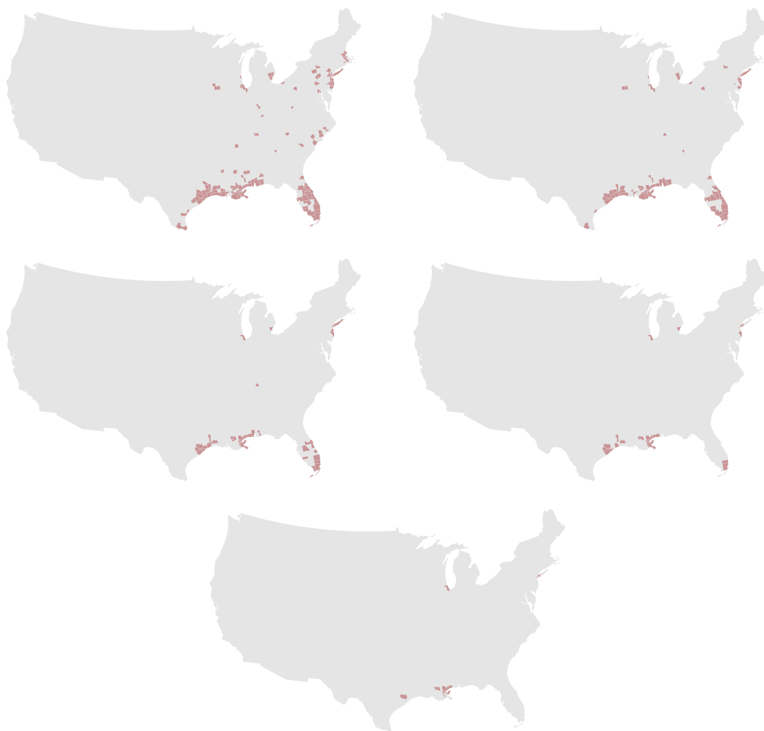
Figure SI-4: Counties impacted by high damage storms —All panels plot counties impacted by high damage storms. For all panels, a county is considered impacted if it meets either the flooding or wind speed threshold. To be considered impacted in the top-left map, a county must have been impacted by at least one storm that caused at least 10 million dollars in damages over our sample period. In the subsequent panels, from left to right, the damage threshold is 20 million dollars, 40 million dollars, 80 million dollars, and 160 million dollars.
